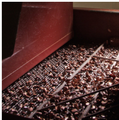
SEPARATION OF COCOA SHELLS FROM COCOA NIBS
